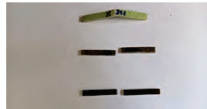
Fig. 4: Short beam Test Specimen after Test
