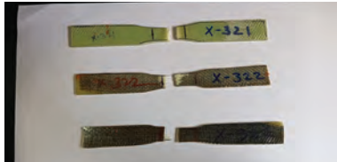
Fig. 1: Tensile Test Specimen after Test
