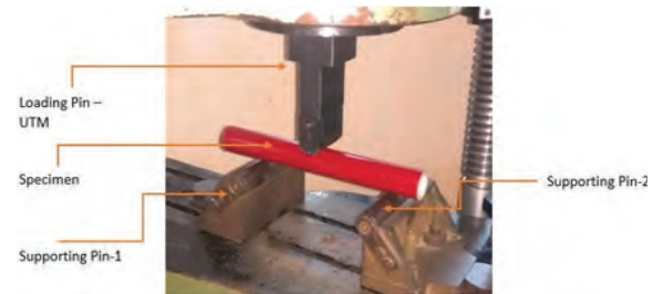
Fig. 9: Three point bending test on sample
