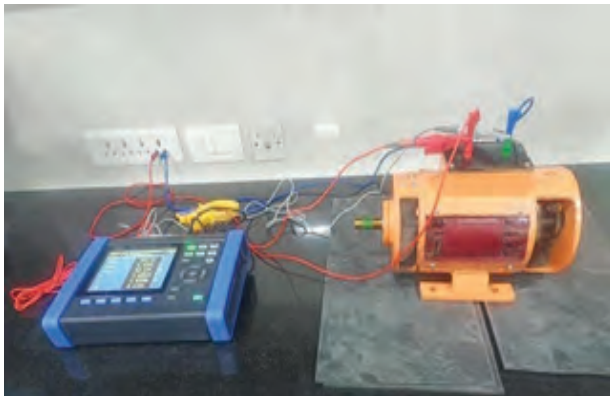
Fig. 3. Grid connected single phase induction motor through power quality analyzer.
