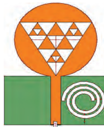
Fig. 7: Modified CM antenna using circular spiral
