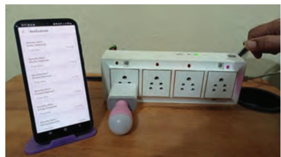
Fig. 15: Smoke Detected Alert
