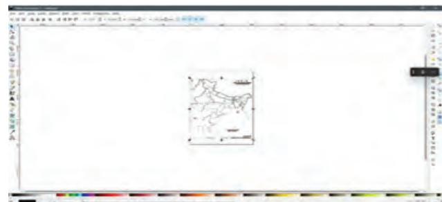
Any image can be converted into graphics code, or G-code, using Inkscape. G-code tools is an open source Inkscape extension that is used to export G-code for usage with CNC machines. It is built in Python. G-code formats are created by integrating Inkscape with the required extension files. (14 - 18) The Inkscape extensions function within the normal Unix IO model, receiving SVG as input on standards and
