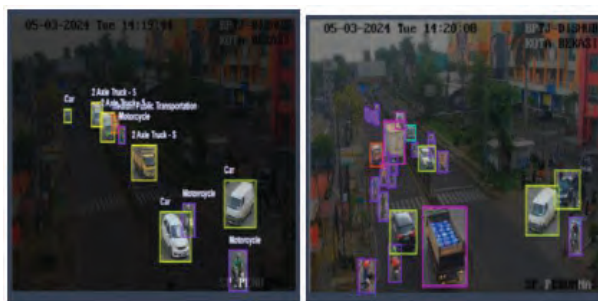
Fig. 4: Training Images with Annotations for different types of Classes [Car, Motorcycle, Truck, Bus etc ]
