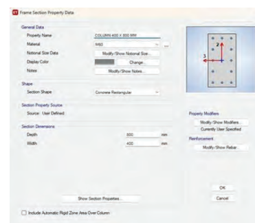
Fig. 1: Column Section Property Data
