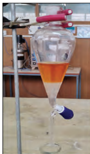
Fig. 4: Water wash of FAME layer
